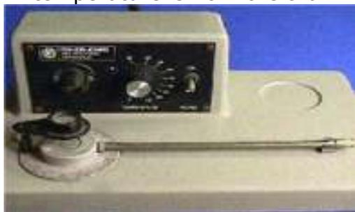
Figure 1. A Fisher-Johns melting point apparatus.
